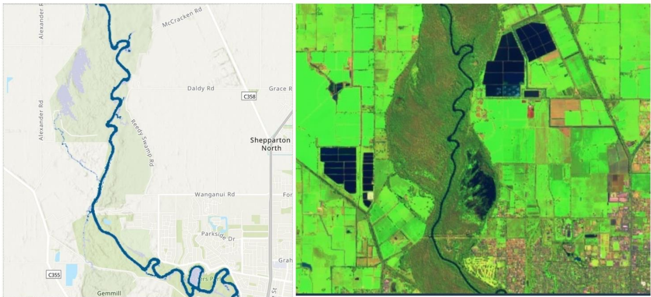
Figure 151 – Comparison of 17,000 ML/d modelled flows at Reedy Swamp (left) and SentinelHub imagery for 12 September 2022 with an average daily flow rate of 17,860 ML/d @ Shepparton on the right (WMIS)
