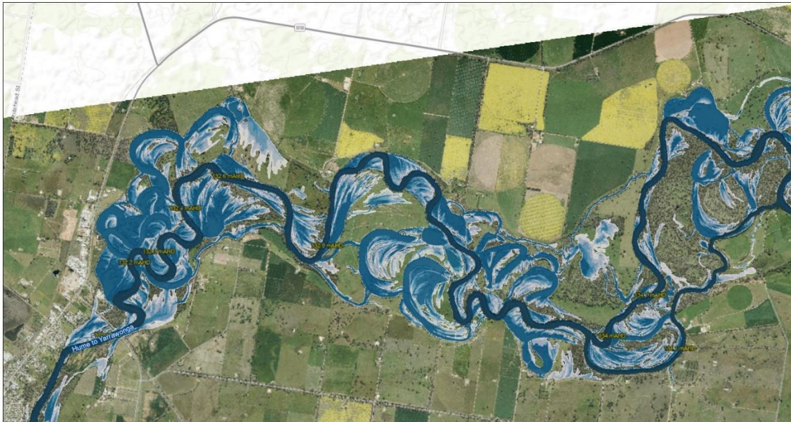
Figure 143 – Murray River upstream of Corowa - Inundation extent of Hume to Yarrawonga flows of 40,000 ML/d
