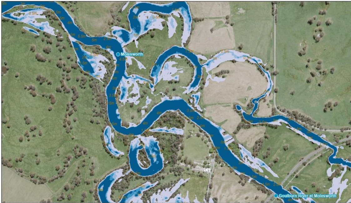
Figure 139 – Goulburn River at Molesworth - Inundation extent at Mid Goulburn flows of 14,000 ML/d
