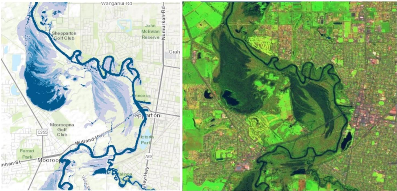
Figure 150 – Comparison of 25,000 ML/d modelled flows at Gemmill Swamp (Lower Goulburn) (left) and SentinelHub imagery for 13 October 2022 with an average daily flow rate of 26,000 ML/d @ Shepparton on the right (WMIS)
