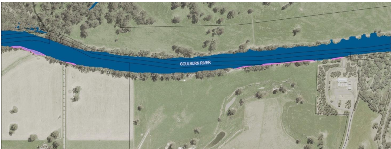
Figure 83 – “Edge effect” examples in Mid Goulburn (pink areas show private land inundation GIS query results)
