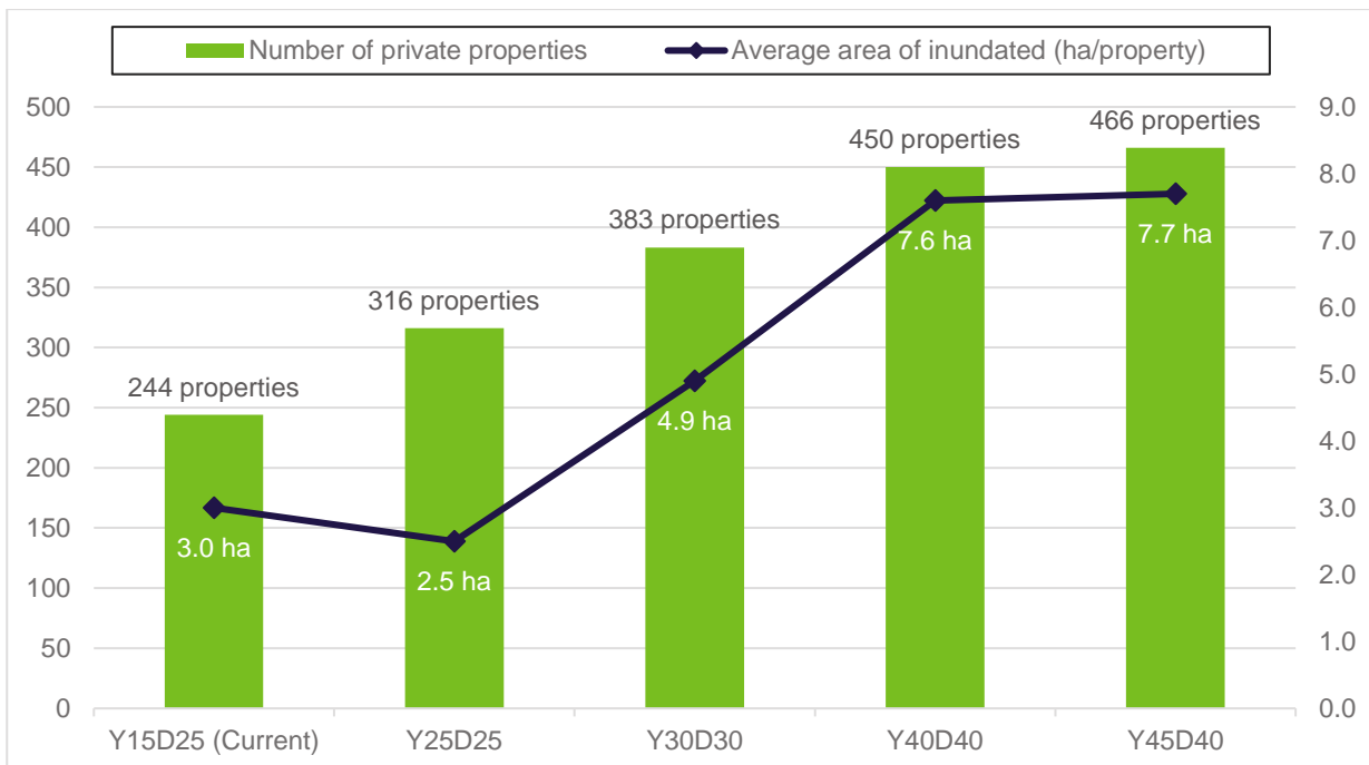
Figure 49 – Murray River Floodplain (Vic Only) - Estimated number of private properties inundated by regulated environmental flow events under modelled relaxed constraint scenarios
