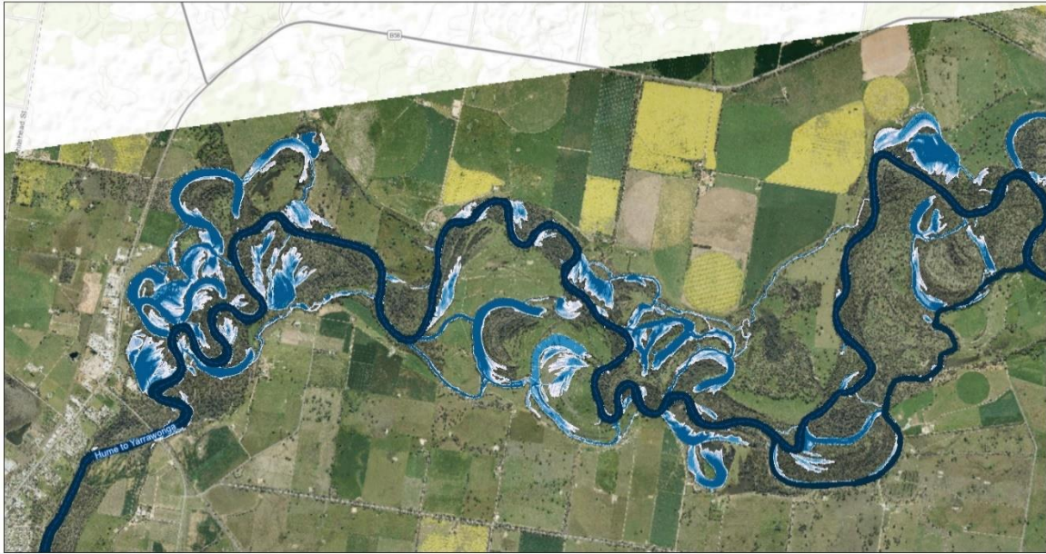
Figure 141 – Murray River upstream of Corowa - Inundation extent of Hume to Yarrowonga flows of 25,000 ML/d
