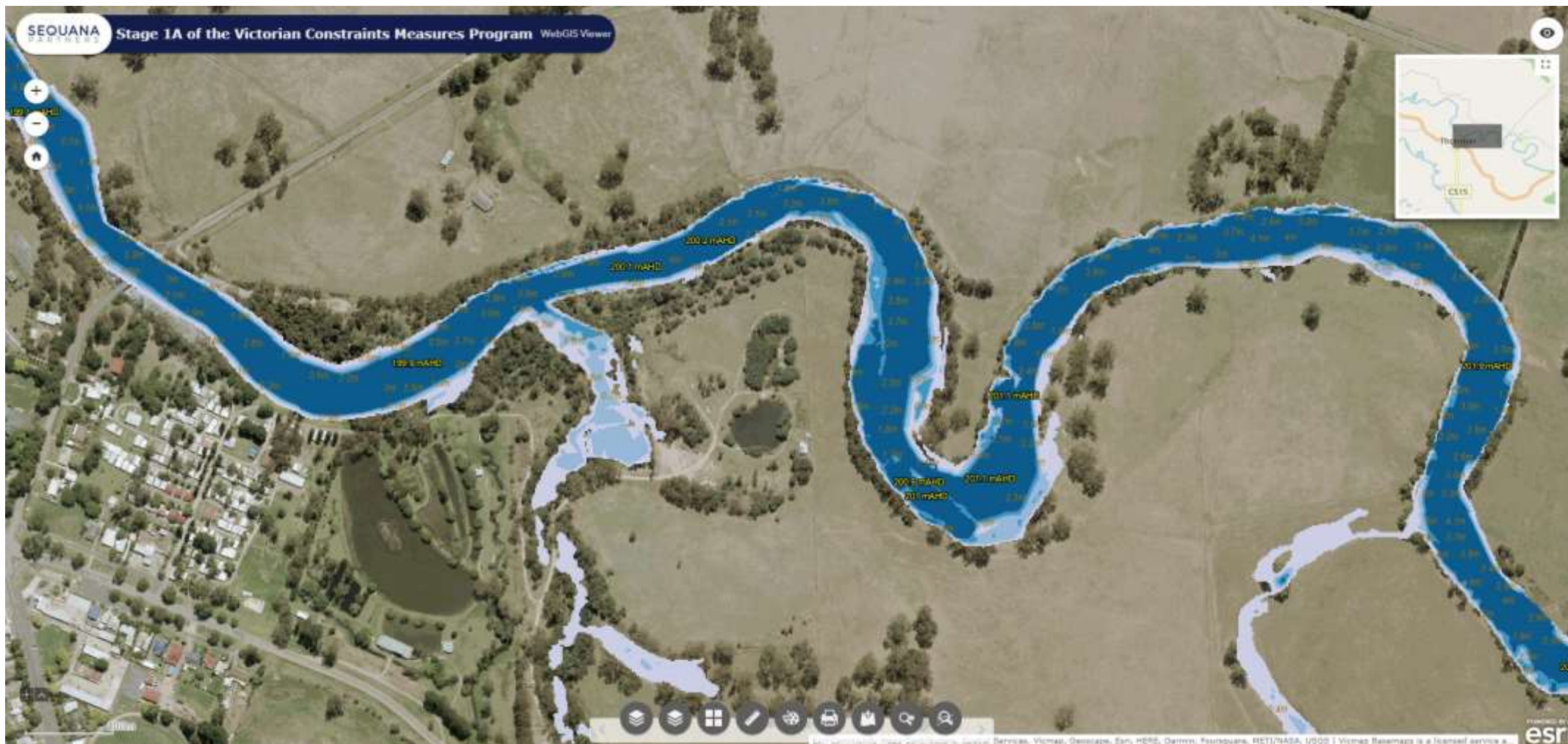
Figure 3: An example of the water level (in m AHD), water depth (in m) and inundation extents simulated by the hydraulic model of the mid-Goulburn. This example shows a section of the Goulburn River upstream of Thornton, at a flow of 12,000 ML/d.
