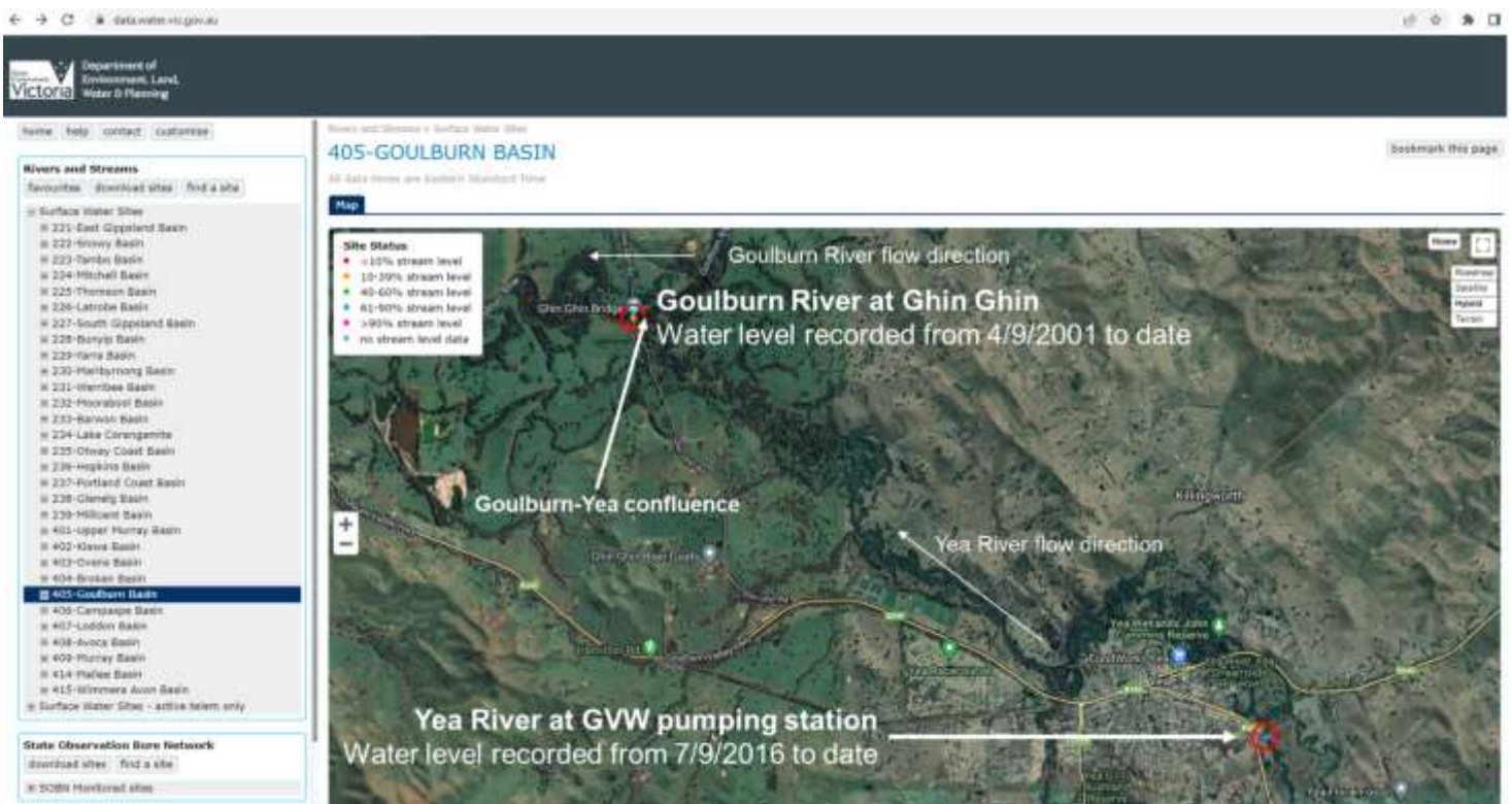
Figure I-1: A screen shot from www.data.water.gov.au showing the location of water level gauges near the Goulburn River – Yea River confluence, and the available period of record.
