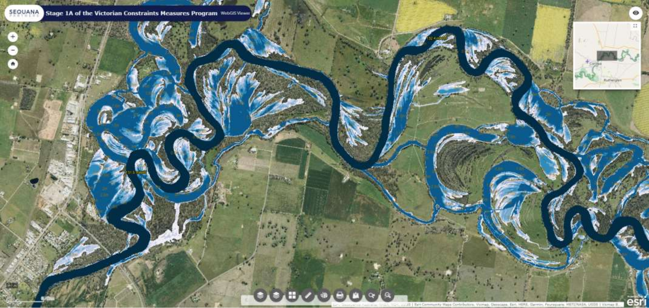
Figure 4: An example of the water level (in m AHD), water depth (in m) and inundation extents simulated by the hydraulic model of the River Murray (Zone 7; Hume to Yarrowonga). This example shows a section of the River Murray upstream of Corowa, at a flow of 30,000 ML/d.
