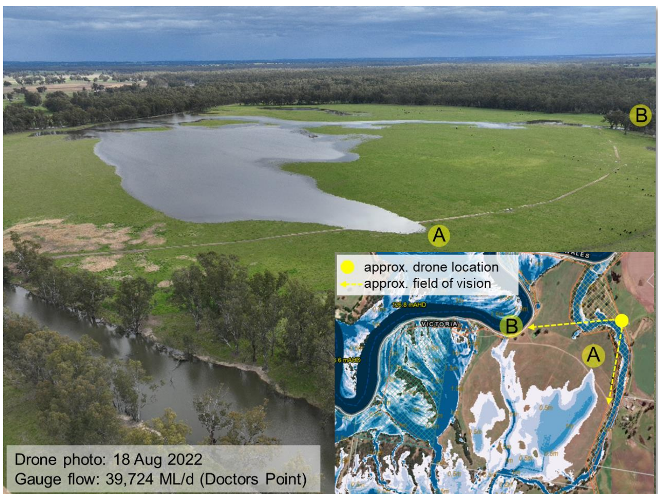
Figure 28: Drone photo taken at Bunyarra with unregulated river flows measuring 39,724 ML/d at Doctors Point (Murray River) on 18 August 2022 and modelled inundation at Bunyarra at flows of 40,000 ML/d
