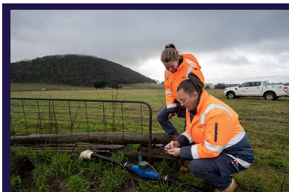
Figure 3. Water corporation field staff reading non-urban meter measuring groundwater use (Dunnstown, Victoria).
