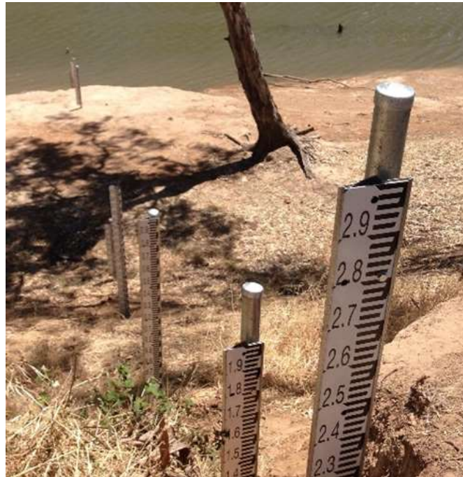
Figure 15 Staff Gauges with backing plates
