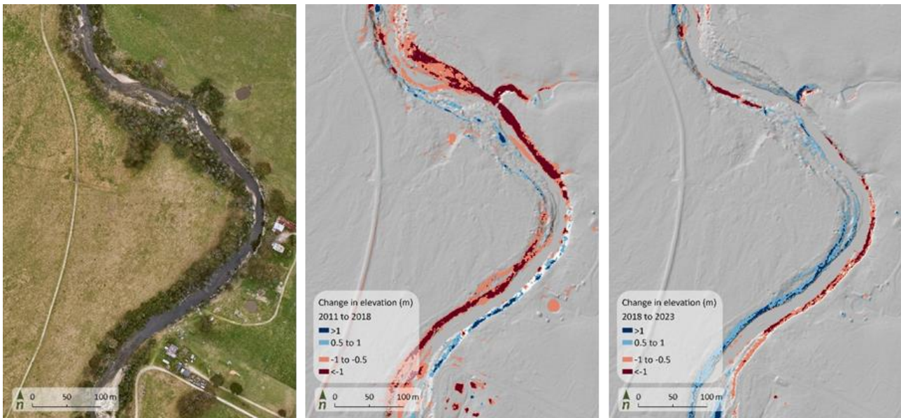
Figure 38. Change in elevation of a meander bend on the Cann River between 2011 and 2018 (middle), and 2018 and 2023 (right).
