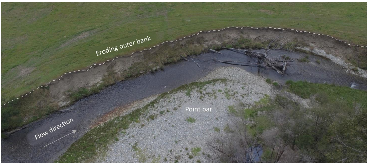
Figure 86. Example of a near vertical upper bank within the study reach (Site 3). Large woody debris is situated along the toe of bank.
