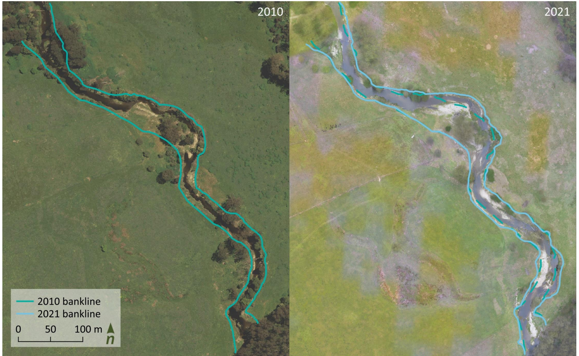
Figure 88. Aerial imagery analysis showing bankline retreat between 2010 (left) and 2021 (right).
